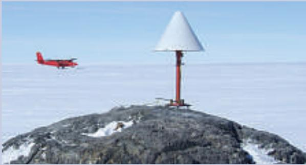
*Global Positioning System measuring glacial isostatic adjustment in West Antarctica.*
